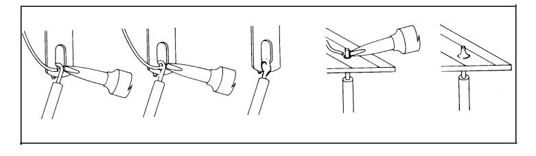
Excess solder may be removed from a connection by heating it and allowing the solder to flow onto the iron, which is then wiped on the sponge.
